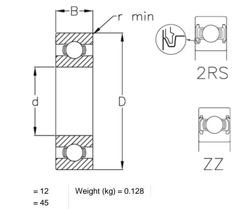
B= 12Wed= 45D= 68Dynamic load C (kN)= 15.1Max rpm greased= 9800Max rpm oil lubricated= 12000r min= 0.6Static load C0 (kN)= 11.2
